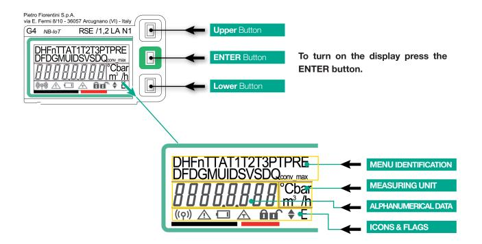
An all-segment lit-up test is performed for a couple of seconds upon display activation, then the Current Index of Converted Volume is shown in cubic meters [m3] with 5 units and 3 decimals.
