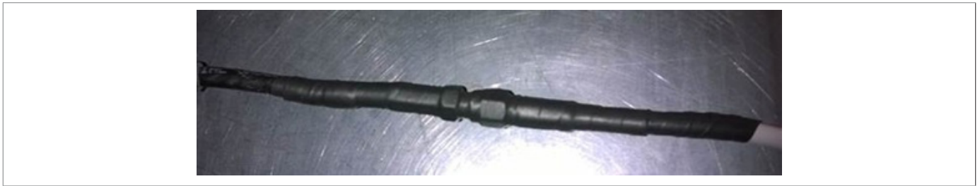
Fig. 7.22. Recommended application method (protection against water infiltration)
